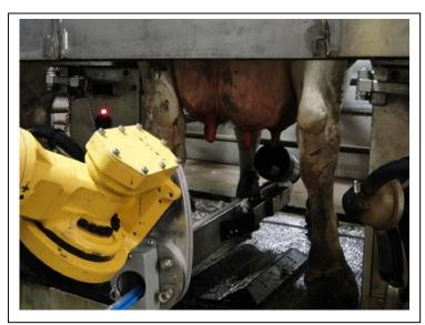
every 8.2 minutes. That means a new cow enters every 6.85 seconds, and it also means a robot applying any work function to every cow has only that much time to work with. This system has proven that teat spraying in that time is possible, and they are working on another arm that sanitizes and preps the udder. Rosendale Dairy, which we visited with Progressive Dairy Operators last June, installed a post dip system on their 80 stall rotary in October. A
