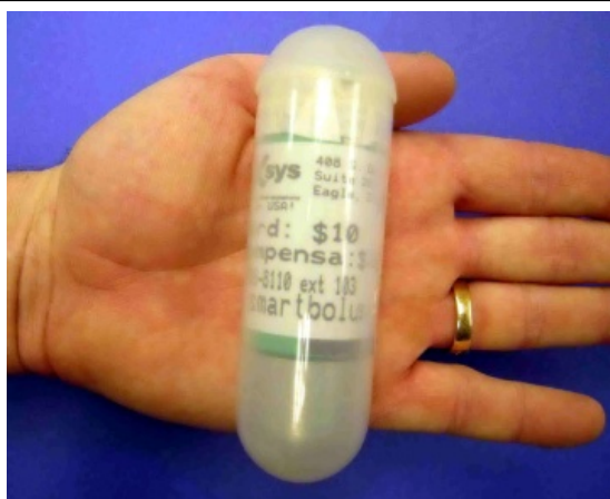
Rumen Temperature Bolus, returnable to the manufacturer for re-charging and re-use
