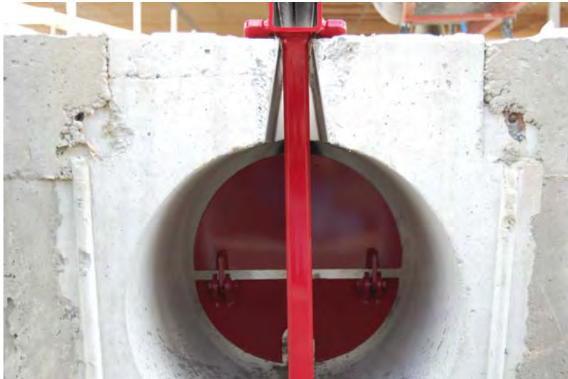
End view of the tube and paddle of a Jamesway tube scraper system.
