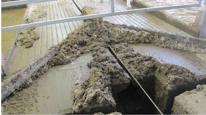
A Norbco tube scraper at Post Dairy in New York State. Note there is very little manure in front of the scraper as it approaches the end of this 340 foot long alley in this 3 robot barn bedded with shavings.
