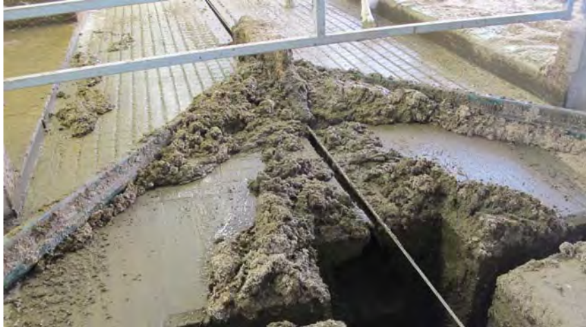
A Norbco tube scraper at Post Dairy in New York State. Note there is very little manure in front of the scraper as it approaches the end of this 340 foot long alley in this 3 robot sand bedded barn.
