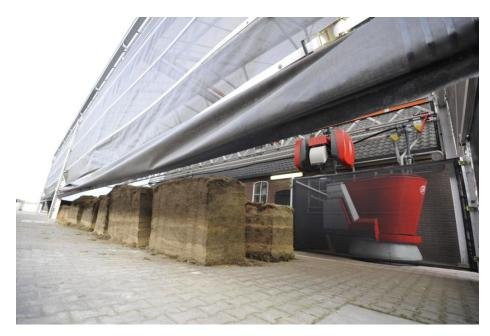
The Vector robotic feed mixing and delivery system, loading forages in the "feed kitchen, using the track mounted grabber. Planning appropriate feed kitchens will be a new aspect of design for barns using these systems.
