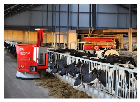
The timing and amount of feed delivered by the Vector is determined by a laser measurement of the amount of feed left at the last push up. Fresh feed can be delivered automatically as many as ten times per day.
